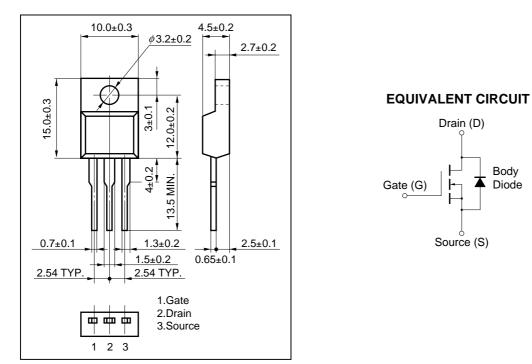
**Remark** Strong electric field, when exposed to this device, can cause destruction of the gate oxide and ultimately degrade the device operation. Steps must be taken to stop generation of static electricity as much as possible, and quickly dissipate it once, when it has occurred.
